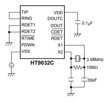
Supply current testing: All, except PDWN and  $\overline{\text{RTIME}},$  unwired pins are left floating.
