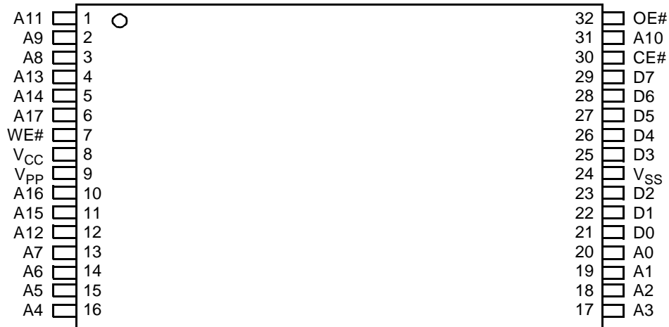
32-Pin TSOP—Standard Pinout
