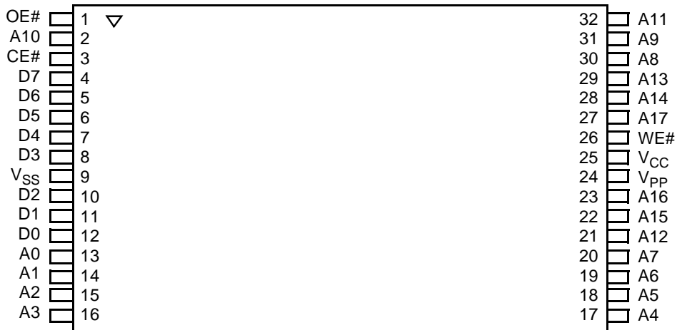
32-Pin TSOP—Reverse Pinout
