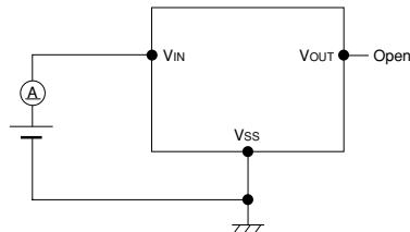
Measuring Circuit 2 : Output Voltage, Oscillation Check, Line Regulation, Dropout Voltage, Load Regulation
