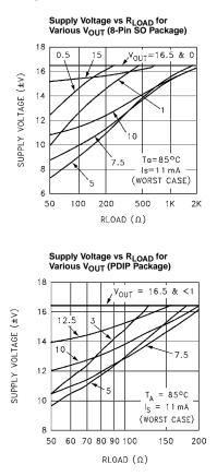
The curves do not include heat removal or forcing air, or the simple fact that the package will probably be attached to a circuit board, which can also provide some form of heat removal. Larger temperature and voltage ranges are possible with heat removal and forcing air past the part.
