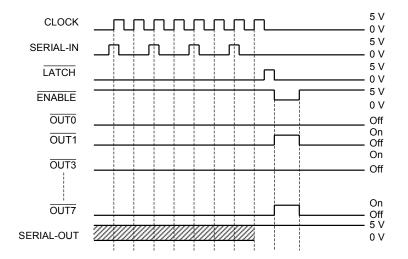
Note: Latches are level-sensitive, not rising edge-sensitive, and are not synchronized with the CLOCK signal. The data will pass through the latch circuit if the latch input is set at "H" level, and will be retained if the input is set at "L".
