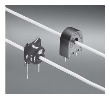
Designed for use above 20 kHz, these sensors function as the secondaries of a current transformer. The conductor carrying the current to be measured is the "one turn primary." Sensitivity can be set at 1 Volt per Ampere or at other desired values. It can also be doubled by looping the conductor through the hole twice. Applications include sensing branch circuit overload, switcher feedback, and detecting load drop or shutdown.
