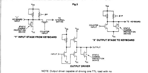
NOTE: Output driver capable of driving one TTL load with no external resistor. Capable of driving two TTL loads using an external 6.8K $\Omega$  resis-
