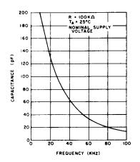
Fig.5 OSCILLATOR FREQUENCY vs. C<sub>2</sub>
