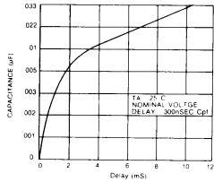
Fig.4 STROBE DELAY vs. C.
