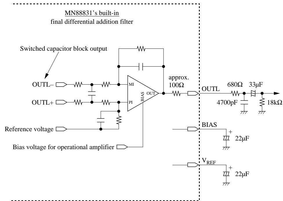
Structure of Analog Post Filter and Sample Analog Connections
