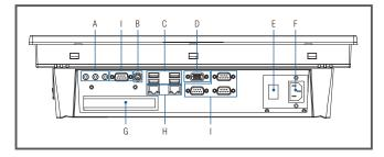
A: Line in/Line out/Mic in B: PS2 Mouse&Keyboard
