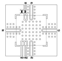
**App Note [1] Biasing** - Please refer to the functional block diagram and pin-out table for biasing information. The device is operated by biasing VD=4.0V with ID=180 mA by adjusting the applied voltage on VG1.VG1 typically requires-0.5V to result in the drain current being 180mA. The nominal input impedance of this gate is 180?, so it should be noted that the nominal gate current will be 2.7mA.
