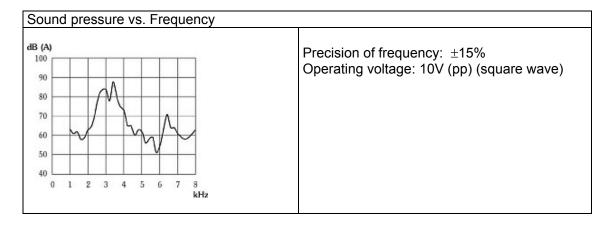
All measurements are made at 30 cm in free air at 21°C.
