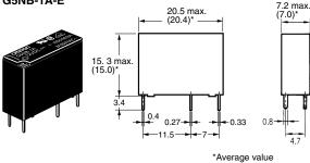
PCB Mounting Holes (Bottom View) Tolerance:  $\pm 0.1 \text{ mm}$
