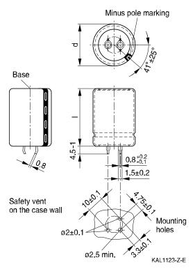
Snap-in terminals, length  $6.3 \pm 1$  mm. Also available in a shorter version with a length of 4.5 - 1 mm. For packing mode and ordering example see next page.
