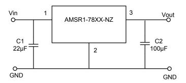
C1: A low ESR capacitor is required to keep the noise of the converter to a minimum.
