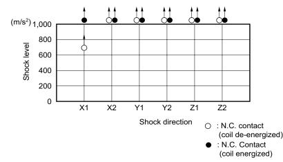
Shock application time : 11 ms, half-sine wave Test material : coil, energized and de-energized Shock direction : set under diagram Detection level : chatter  $\geq$  100 µs
