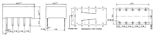
AL-D type (Double winding latching type)
