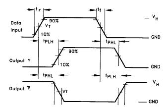
Input and output threshold voltage:  $V_T = 50\%$  Vcc for AC; 1.5V for ACT  $V_H = V_{CC}$  for AC, 3V for ACT
