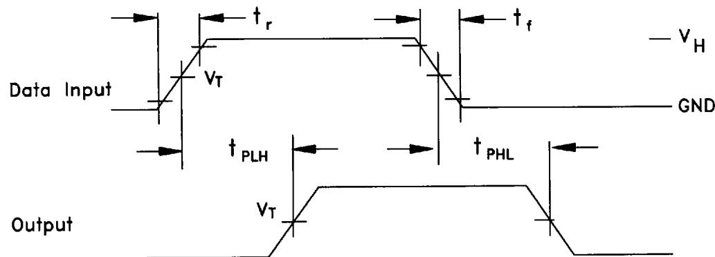
Input and output threshold voltage:
