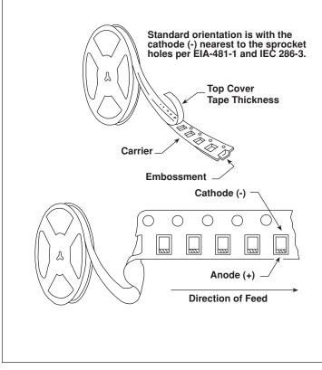
**Tape and Reel Specifications**: All case codes are available on plastic embossed tape per EIA-481-1. Tape reeling per IEC 286-3 is also available. Standard reel diameter is 13" [330mm]. 7" [178mm] reels are available.
