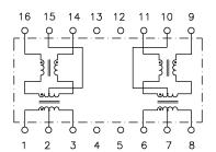
Electrical Specifications @ 25°C CMR (0.1-100MHz): -40dB typ Operating Temp: -40 to +85°C Crosstalk (0.1-100MHz): -40dB min
