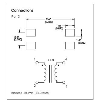
Dimensions shown are in millimetres (inches). Terminal plating JESD97 category = e2. Recommended reflow solder profile: 2 minutes @ 150-200°C, 10 seconds @ 260°C; time above 217°C 60 seconds maximum.
