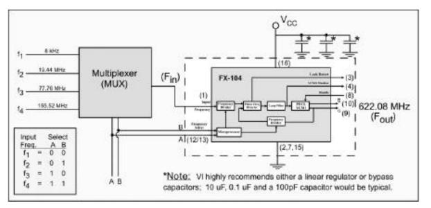
All components outside the dotted line box are user supplied components. This is just one possible configuration of the FX-104. For additional information about your specific needs, please contact our factory.
