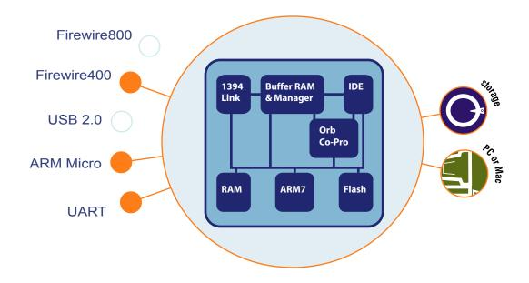
**The Oxford 911** plus is the latest generation 1394A to ATA7/ATAPI (IDE) bridge. It supports all PIO, DMA and UDMA modes up to UDMA6, delivering a sustained data transfer performance of over 40MBytes/sec. Hardware features include SBP2.0 acceleration with 'fast start', in addition to dual disk striping and transparent spanning capabilities, all designed to achieve maximum data throughput.
