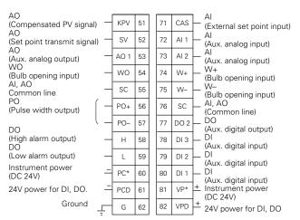
Note \* Symbols for AC power supply are VPO, PCO. Output is 24V DC (0.1A max.) approx.
