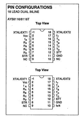
frequency  $(f_x)$  is used by the 8136/8136T to provide a high frequency output  $(f_x/4)$ .
