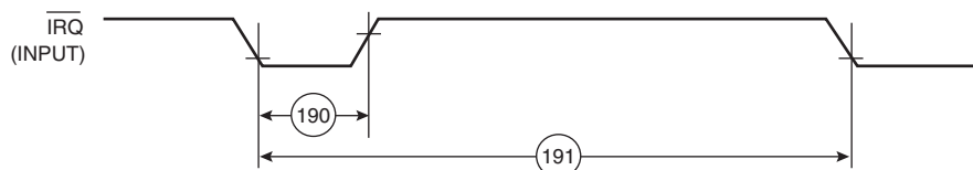
Figure 20. Interrupts Timing Diagram
