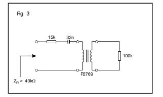
At the expense of a small loss, (approximately 1.5dBV) the circuit in fig. 3 provides an impedance exceeding  $40k\Omega$ , 200Hz - 4.3kHz, and frequency response flatness within ±0.25dB over the same band.
