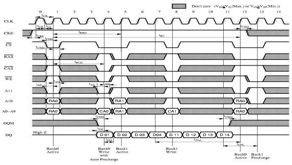
$RA0/l: Row\ Address\ (Bank\ 0/l),\quad CA0/l: Column\ Address\ (Bank\ 0/l),\quad Q0 \times /l \times : Output\ Data\ (Bank\ 0/l)$
