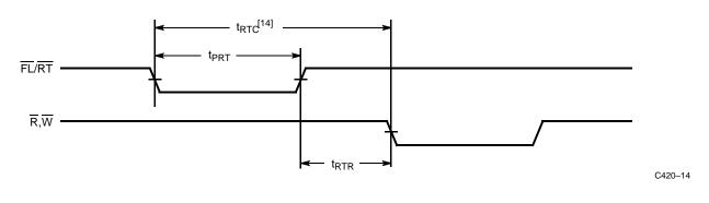
Notes: 13.  $\overline{EF}$ ,  $\overline{HF}$  and  $\overline{FF}$  may change state during retransmit as a result of the offset of the read and write pointers, but flags will be valid at t<sub>RTC</sub>. 14.  $t_{RTC} = t_{PRT} + t_{RTR}$ .
