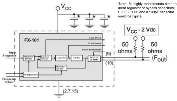
All components outside the dotted line box are user supplied components and/or connections. This is just one possible configuration of the FX-101. For additional information about your specific needs please contact our Factory.
