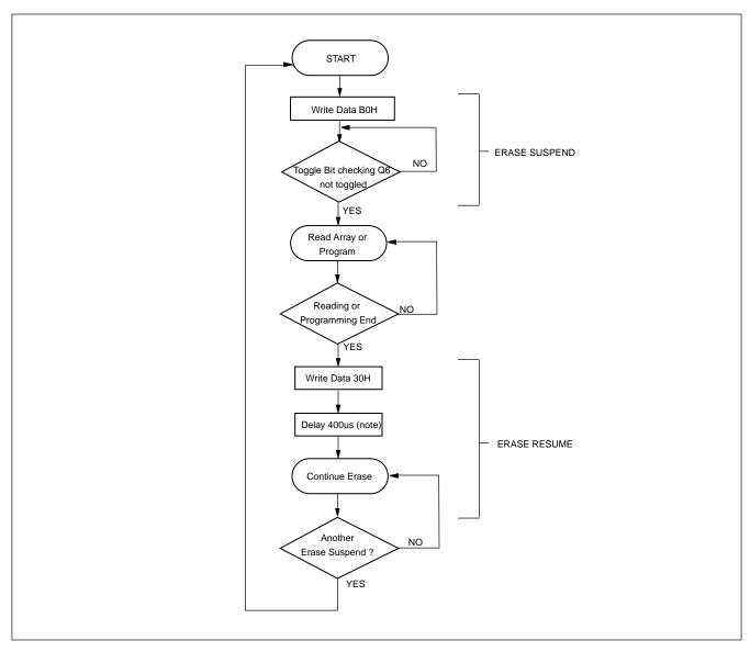
Note: If the system implements an endless erase suspend/resume loop, or the number of erase suspend/resume is exceeded 1024 times, then the 400us time delay must be put into consideration.
