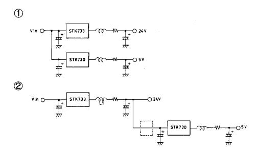
(Note) Due to the negative influences the 24 V system receives from the STK730 input ripple current and the assertion of L1, L should be installed in the [\_\_\_\_] section and the formation of a LC filter.
