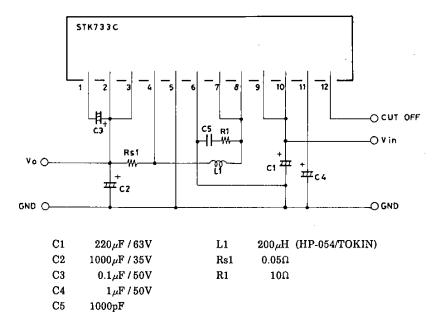
Note) Since the 5 pin is grounded to the substrate, these are influenced by noise when the radiator is connected to the circuit of the FG and GND lines. Under such conditions, the radiator should either be floated or an insulated seating used.
