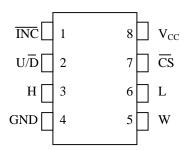
8-Pin DIP (300-mil) 8-Pin SOIC (150-mil) 8-Pin uSOP (118-mil) 8-Pin Flip Chip Package
