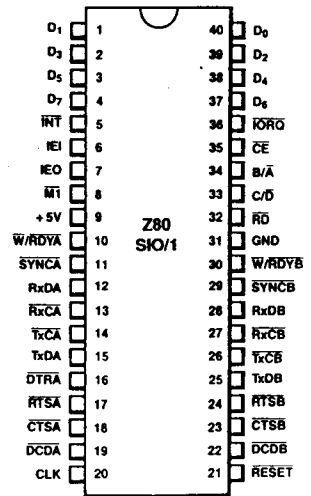
Figure 4. 40-pin Dual-In-Line Package (DIP), Pin Assignments
