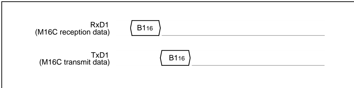
Figure 1.32.39. Timing of baud rate 19200
