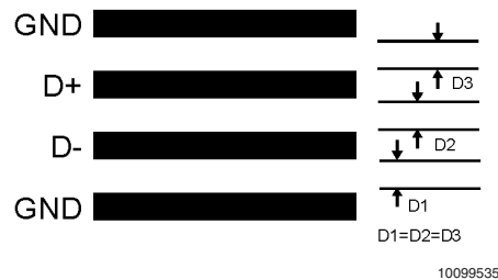
FIGURE 9. Recommended Diode Trace Layout
