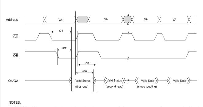
VA=Valid address; not required for Q6. Figure shows first two status cycle after command sequence, last status read cycle, and array data read cycle.
