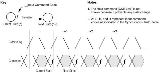
Current State and Next State Definition for Pipelined and Flow through Read/Write Control State Diagram
