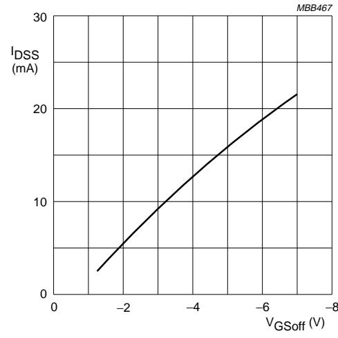
$V_{DS} = 15 V; T_j = 25^\circ C$ .
