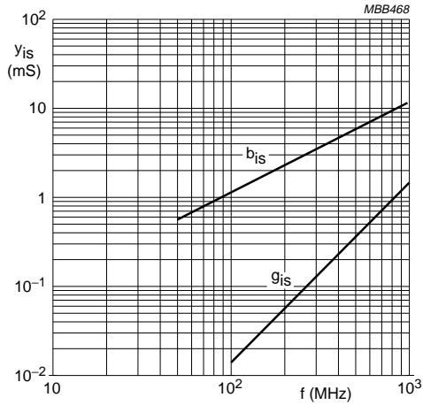
$V_{DS} = 10$  V;  $I_D = 1$  mA;  $T_{amb} = 25$  °C.
