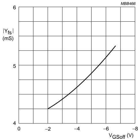
$V_{DS} = 15 V; V_{GS} = 0; T_j = 25^\circ C$ .
