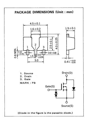
The 2SJ197, P-channel vertical type MOS FET, is a switching device which can be driven directly by the output of ICs having a 5 V power source.
