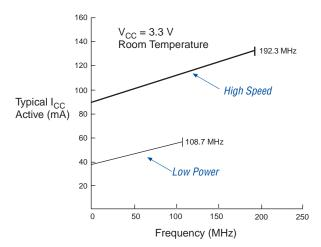
Figure 13. I<sub>CC</sub> vs. Frequency for MAX 7000A Devices (Part 2 of 2)
