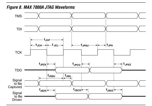
Figure 8 shows timing information for the JTAG signals.
