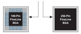
100-Pin FineLine BGA Package (Reduced I/O Count or Logic Requirements) 256-Pin FineLine BGA Package (Increased I/O Count or Logic Requirements)
