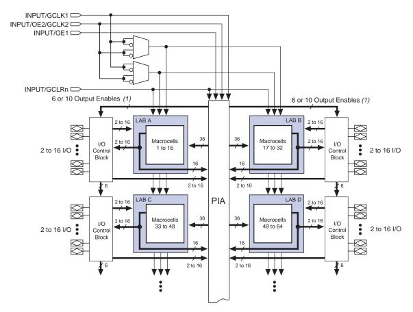
Figure 1. MAX 7000A Device Block Diagram
