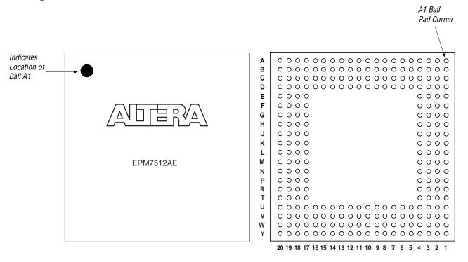
Figure 23. 256-Pin FineLine BGA Package Pin-Out Diagram
