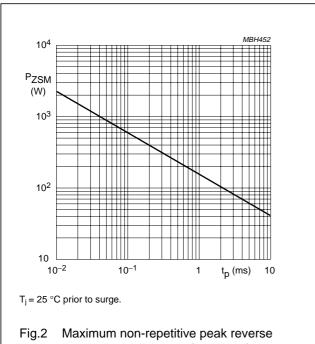
Fig.2 Maximum non-repetitive peak reverse power dissipation as a function of pulse duration (square pulse).
