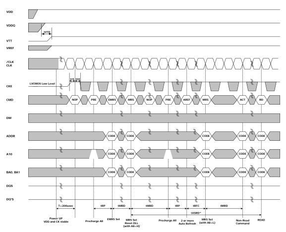
$^{\star}$  200 cycle(tXSRD) of CK are required (for DLL locking) before Read Command
