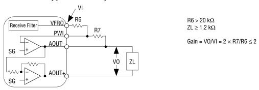
During power saving and power down modes, the outputs of AOUT+ and AOUT- are in a high impedance state.
