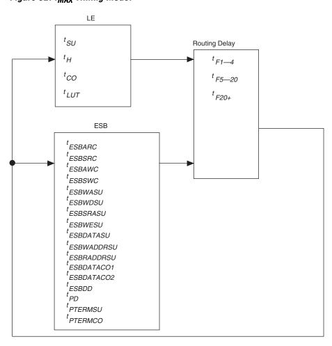
Figure 32. f<sub>MAX</sub> Timing Model
