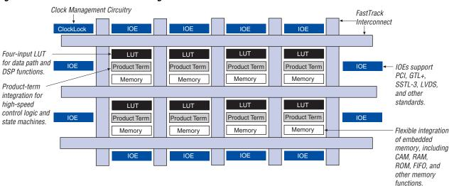
Figure 1. APEX 20KC Device Block Diagram
