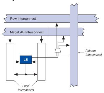
Figure 11. Driving the FastTrack Interconnect
