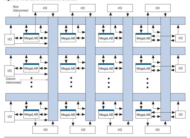
Figure 9. APEX 20KC Interconnect Structure
