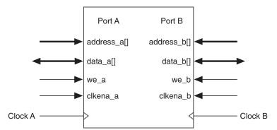
Figure 19. APEX 20KC ESB Implementing Dual-Port RAM
