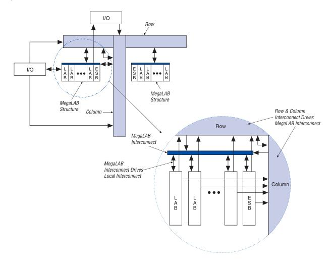
Figure 10. FastTrack Connection to Local Interconnect
