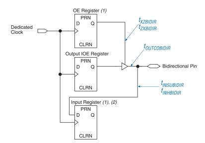
Figure 35. Synchronous Bidirectional Pin External Timing
