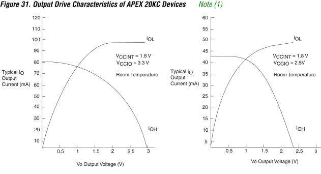
Figure 31. Output Drive Characteristics of APEX 20KC Devices
