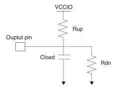
Figure 37. AC Test Conditions for SSTL-3 Class I & II I/O Standards
