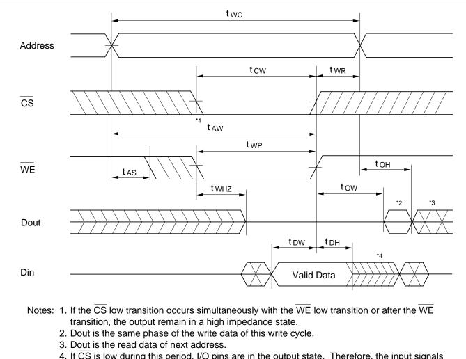
Write Timing Waveform (2) (OE Low Fixed)
