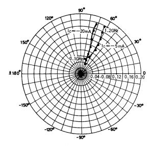
$S21e: V_{CE} = -10V \\ f = 100MHz, 200 \text{ to } 1200MHz \text{ (200MHz step)}$
