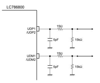
\* The value of resistors and capacitors in this circuit might be needed to be adjusted for each application.
