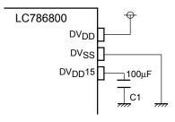
\* Same circuit need to be mounted both for two regulator pins. (No.44 and No.90)
