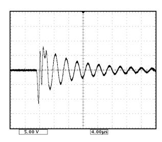
Unloaded high voltage output 4 us/div 5 kV/div
