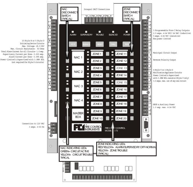
Mounting Location for ZDM-FC73 or FC-5280 (ZDM-FC73 can mount remotely in FC-2190 Accessory Cabinet)
